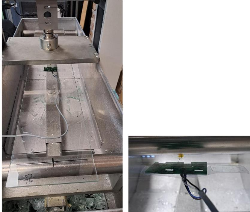
Fig. 1 Experimental set-up with the detail of strain gauges for indirect displacement measurement
