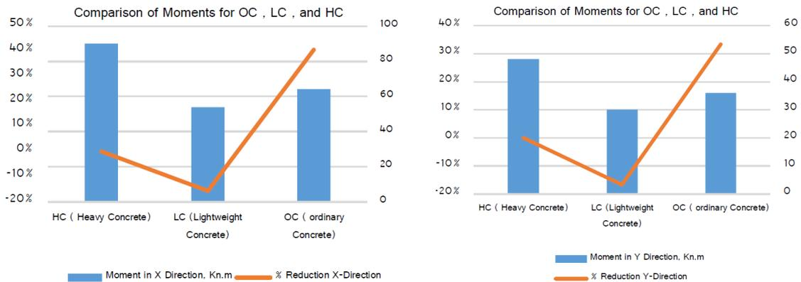
Fig. 11 Bending moment for slabs (OC, LC, and HC)
