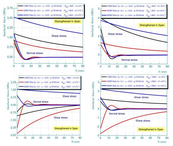
Fig. 8 Effect of the rigidity of composite plate on interfacial stresses for a continuous RC damaged beam Strengthened with presstressed composite plate: Strengthened in span
