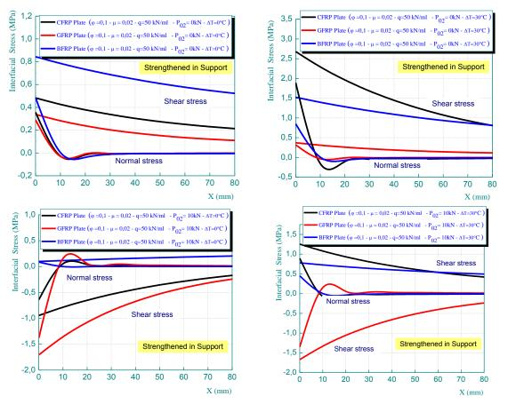
Fig. 9 Effect of the rigidity of composite plate on interfacial stresses for a continuous RC damaged beam strengthened with presstressed composite plate: Strengthened in support
