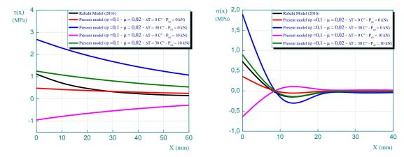
Fig. 7 Variations of interfacial stresses in RC damaged continuous beam strengthening with prestressed laminate plate: Comparison between the analytical model "Strengthened in support: Upper part"
