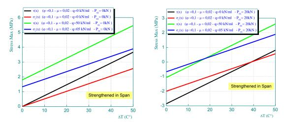
Fig. 10 Effect of temperature variation on interfacial stresses for a continuous RC damaged beam strengthened with presstressed composite plate: Strengthened in span
