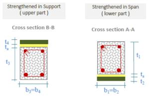
Fig. 2 Continuous damaged reinforced concrete beam bonded with a prestressed composite plate: cross section in span and cross in support
