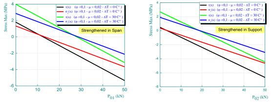
Fig. 12 Effect of the prestressing force of composite plate on interfacial stresses for a continuous RC damaged beam strengthened with presstressed composite plate
