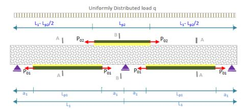
Fig. 1 Damaged reinforced concrete continuous beam bonded with a prestressed composite plate
