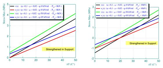
Fig. 11 Effect of temperature variation on interfacial stresses for a continuous RC damaged beam strengthened with presstresed composite plate: Strengthened in support
