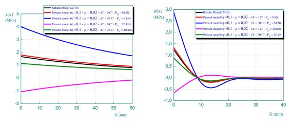
Fig. 6 Variations of interfacial stresses in RC damaged continuous beam strengthening with prestressed laminate plate: Comparison between the analytical model "Strengthened in span: Lower part"
