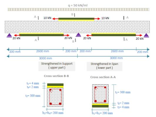
Performance of damaged RC continuous beams strengthened by prestressed laminates plate... 173
