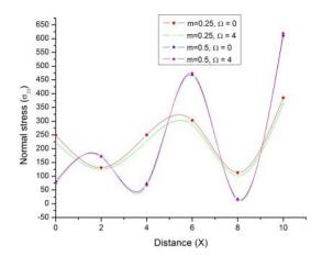
Fig. 5 Variation of normal stress  $\sigma_{33}$  with distance *x* (linearly distributed thermal source)
