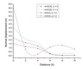
Fig. 7 Variation of normal displacement w with distance x (concentrated thermal source)
