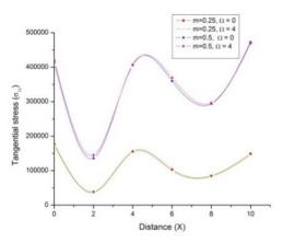
Fig. 4 Variation of tangential stress  $\sigma_{31}$  with distance *x* (linearly distributed thermal source)
