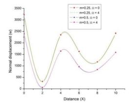
Fig. 2 Variation of normal displacement w with distance x (linearly distributed thermal source)
