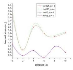
Fig. 15 Variation of normal stress  $\sigma_{33}$  with distance *x* (linearly distributed mechanical force)
