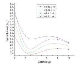
Fig. 10 Variation of Normal stress  $\sigma_{33}$  with distance x (concentrated thermal source)
