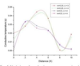
Fig. 3 Variation of conductive temperature  $\phi$  with distance *x* (linearly distributed thermal source)
