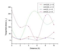
Fig. 14 Variation of tangential stress  $\sigma_{13}$  with distance *x* (linearly distributed mechanical force)
