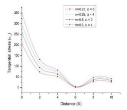
Fig. 9 Variation of tangential stress  $\sigma_{31}$  distance *x* (concentrated thermal source)
