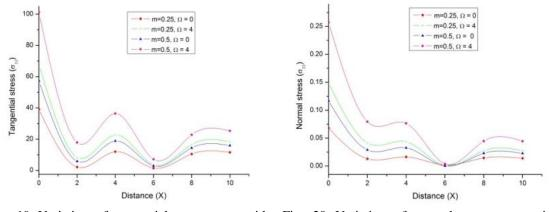
Fig. 19 Variation of tangential stress  $\sigma_{13}$  with Fig. 20 Variation of normal stress  $\sigma_{33}$  with distance *x* (concentrated mechanical force) distance *x* (concentrated mechanical force)
