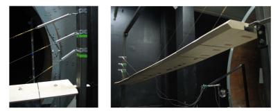
Fig. 3 The bridge model mounted in the wind tunnel
