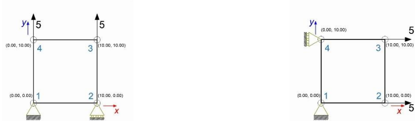
(c) Concentrated traction force on y direction (variant A) (d) Concentrated traction force on x direction (variant B)
