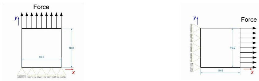
(a) Traction force applied on y direction (variant A) (b) Traction force applied on x direction (variant B)
