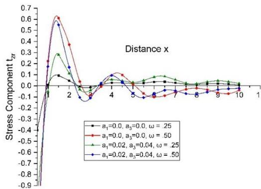
Fig. 12 Variations of the stress component  $t_{zr}$  with distance x
