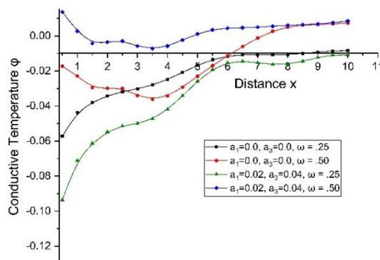
Fig. 22 Variations of temperature  $\phi$  with distance  $x$
