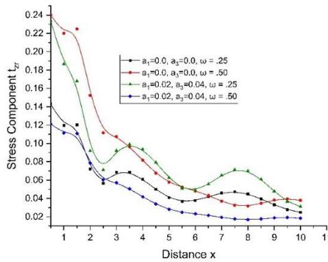
Fig. 18 Variations of the stress component  $t_{zr}$  with distance  $x$
