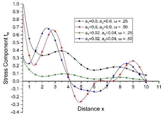
Fig. 5 Variations of stress component  $t_{rr}$  with distance  $x$
