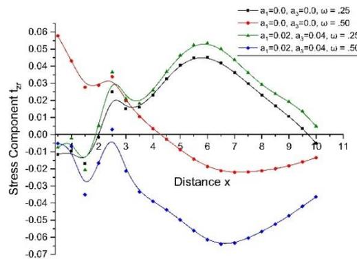
Fig. 24 Variations of the stress component  $t_{zr}$  with distance x
