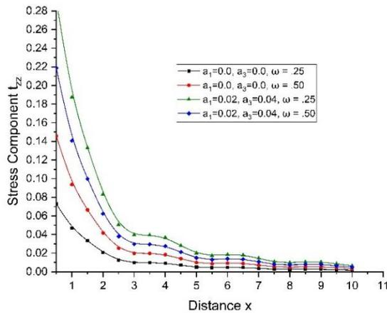
Fig. 7 Variations of the stress component  $t_{zz}$  with distance  $x$
