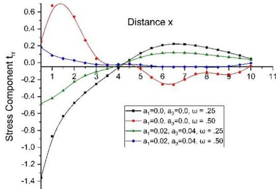
Fig. 11 Variations of stress component  $t_{rr}$  with distance x
