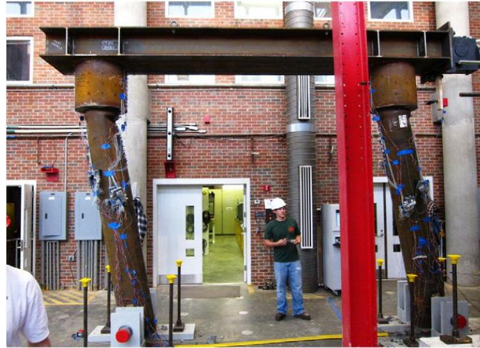
Fig. 7 Deformed shape of the experimental specimen (Fulmer et al. 2015)
