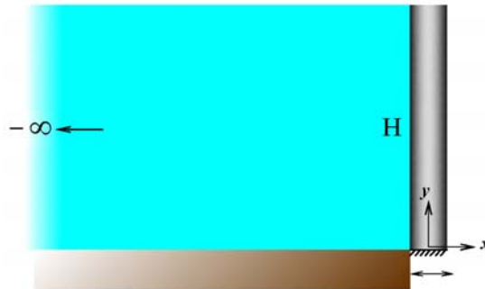
Fig. 1 A two-dimensional slender beam–water interaction system subjected to a horizontal ground acceleration
