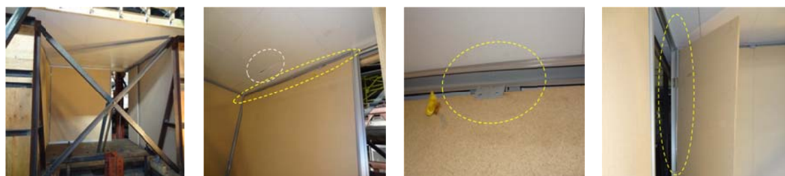
(a) Set-up before testing (b) Panel dislocation and wall damage (c) Shearing-off of the top wall brackets (d) Damage to the door top hinge
