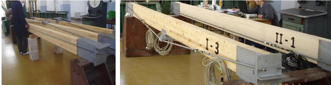
(a) The installation of cables on models of Series I (b) models of hybrid girders for testing
