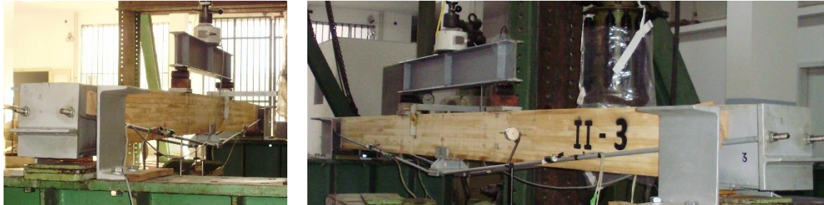
(a) deflection of glued laminated girder of prestressing force is increased due to an increase in the percentage of moisture content (b) deflection of prestressed hybrid system of external loads on condition of moist wood beam
