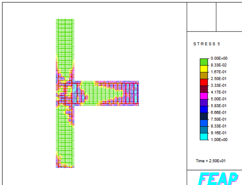
Fig. 14 Damage distribution on specimen LH11 (HIGH confinement) for a displacement of 3.5 inches
