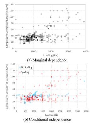
Fig. 3 Marginal vs. conditional association between the compressive strength of concrete and loading in fire-exposed RC columns
