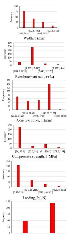
Spalling (left=column does not spall, right=column spalls Fig. 10 Frequency of identified features of selected RC columns in the compiled database
