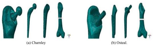
Fig. 2 Finite element meshes of hip prosthesis components
