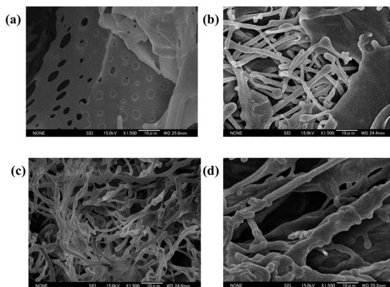
Fig. 1 SEM images of the freeze-dried polymers (Scale bar, 10  $\mu\text{m}$ ): (a) Poly(HEAA), (b) PH<sub>99</sub>T<sub>11</sub>, (c) PH<sub>92</sub>T<sub>9</sub>, (d) PH<sub>99</sub>T<sub>52</sub>
