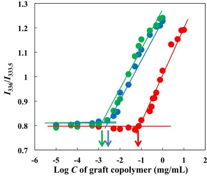
Fig. 5 Plot of  $I_{336}/I_{333.5}$  (from the pyrene excitation spectra) versus  $\log C$ , where  $C$  is the concentration of the graft copolymers. PH<sub>99</sub>T<sub>11</sub>: ●, PH<sub>92</sub>T<sub>9</sub>: ●, PH<sub>99</sub>T<sub>52</sub>: ●
