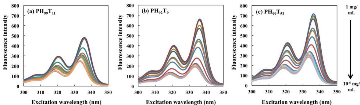
Fig. 4 Excitation spectra of pyrene ( $6.0 \times 10^{-7}$  mol/L) as a function of polymer concentration ( $10^{-5}$ –1 mg/mL) in aqueous solution at 25 °C. (a) PH<sub>99</sub>T<sub>11</sub>, (b) PH<sub>92</sub>T<sub>9</sub>, (c) PH<sub>99</sub>T<sub>52</sub>
