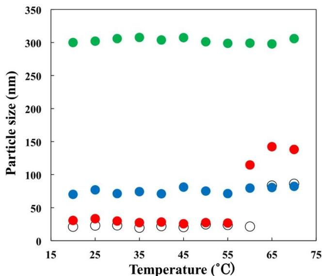
Fig. 3 Change in particle size over the temperature range 20 to 70°C. Poly(HEAA):  $\circ$ , PH<sub>99</sub>T<sub>11</sub>:  $\bullet$ , PH<sub>92</sub>T<sub>9</sub>:  $\bullet$ , PH<sub>99</sub>T<sub>52</sub>:  $\bullet$
