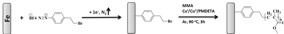
Scheme 3 Schematic illustration of the successive modification steps of the stainless steel (SS) stents [MMA, methyl methacrylate]
