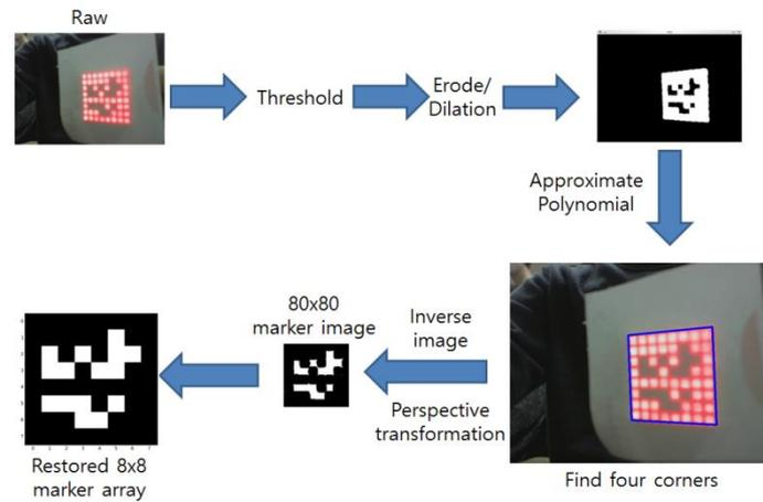
Fig. 2 Overall image processing algorithm for marker detection.
