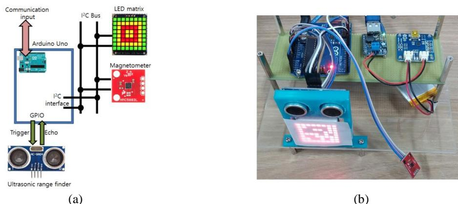
Fig. 1 (a) Circuit diagram of an active marker node. GPIO stands for General Purpose Input and Output. The magnetometer and ultrasonic range finder were used for checking the robot proximity and (b) Image of the developed marker node
