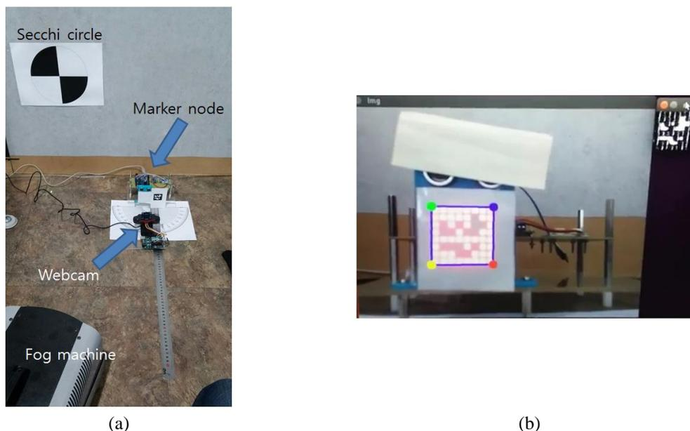
Fig. 3 (a) Experimental setup. (b) Image acquisition and marker recognition under clear bright situation
