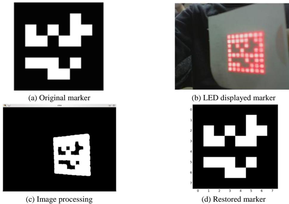
Fig. 4 Restoration of the marker from LED marker. (a) Original AprilTag marker image, (b) LED displayed marker, (c) Contour image of the marker detected during image processing and (d) Restored marker from an inverted contour image, which is identical to the original marker
