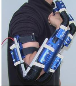
Fig. 25 ASSIST wearable device for weak muscular power for forearm and hand
