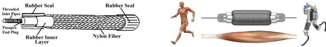
Fig. 14 Pneumatic muscle actuator (Bowler *et al.* 1996, Anon 2010)
