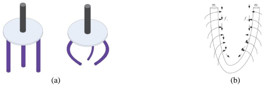
Fig. 11 (a) Schematic of the model and (b) the bending moment profile upon SMA actuation
