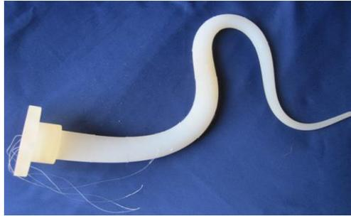
Fig. 31 Tendon driven octopus arm prototype
