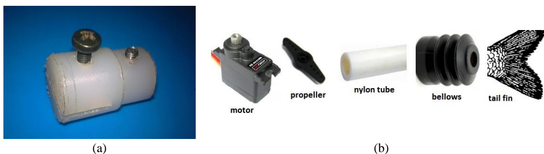
Fig. 4 Representation of the nylon accessory (a) and components of the tail fin mechanism structure (b)
