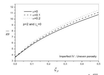
Fig. 24 Variation of the nondimensional fundamental frequency  $\overline{\omega} = \frac{\omega L^2}{h} \sqrt{\frac{\rho_m}{E_m}}$  of FG beam with shear foundation parameter  $\xi_p$  and porosity coefficient  $\alpha$
