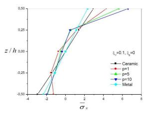
Fig. 9 Non-dimensional axial stress through the thickness (L/h = 5, non-dimensional elastic foundation parameters are :  $\xi_w = 0.1$  and  $\xi_p = 0$ )
