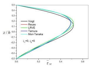
Fig. 15 Variation of the transverse shear stress  $\overline{\tau}_{xz}$  through-the-thickness of a FG beam for different micromechanical models (L/h = 2, p = 1)
