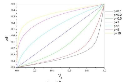
Fig. 2 Functionally graded function  $V_c = \left(\frac{z}{h} + \frac{1}{2}\right)^p$  through the thickness of a FGM beam for different values of the index (p)
