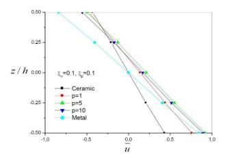
Fig. 7 Non-dimensional axial displacement through the thickness (L/h = 5, non-dimensional elastic foundation parameters are :  $\xi_w = 0.1$  and  $\xi_p = 0.1$ )
