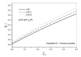
Fig. 20 Variation of the nondimensional fundamental frequency  $\overline{\omega} = \frac{\omega L^2}{h} \sqrt{\frac{\rho_m}{E_m}}$  of FG beam with Winkler parameter  $\xi_w$  and porosity coefficient  $\alpha$
