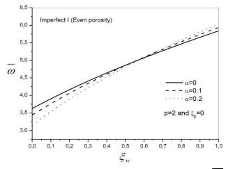
Fig. 17 Variation of the nondimensional fundamental frequency  $\overline{\omega} = \frac{\omega L^2}{h} \sqrt{\frac{\rho_m}{E_m}}$  of FG beam with Winkler parameter  $\xi_w$  and porosity coefficient  $\alpha$
