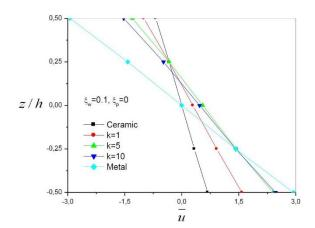
Fig. 6 Non-dimensional axial displacement through the thickness (L/h = 5, non-dimensional elastic foundation parameters are :  $\xi_w = 0.1$  and  $\xi_p = 0$ )
