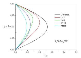
Fig. 13 Non-dimensional transverse shear stress through the thickness (L/h = 5, non-dimensional elastic foundation parameters are :  $\xi_w = 0.1$  and  $\xi_p = 0.1$ )
