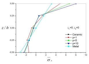
Fig. 8 Non-dimensional axial stress through the thickness (L/h = 5, non-dimensional elastic foundation parameters are :  $\xi_w = 0$  and  $\xi_p = 0$ )
