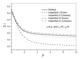
Fig. 25 Variation of non-dimensional frequency  $\overline{\omega}$  of embedded perfect and imperfect FG beams versus volume fraction indices p ( $\alpha = 0.2$  and L/h = 5)
