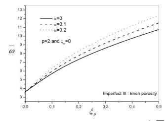
Fig. 23 Variation of the nondimensional fundamental frequency  $\overline{\omega} = \frac{\omega L^2}{h} \sqrt{\frac{\rho_m}{E_m}}$  of FG beam with shear foundation parameter  $\xi_p$  and porosity coefficient  $\alpha$
