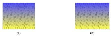
Fig. 3 Porosity models: (a) Evenly distributed porosities; (b) Unevenly distributed porosities
