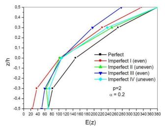
Fig. 4 Variation of Young's modulus E(z) through the thickness of embedded perfect and imperfect FG beams (p = 2 and  $\alpha = 0.2$ )
