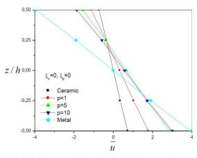
Fig. 5 Non-dimensional axial displacement through the thickness (L/h = 5, non dimensional elastic foundation parameters are:  $\xi_w = \xi_p = 0$ )
