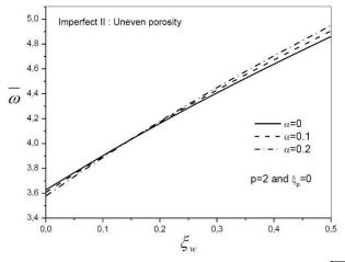
Fig. 18 Variation of the nondimensional fundamental frequency  $\overline{\omega} = \frac{\omega L^2}{h} \sqrt{\frac{\rho_m}{E_m}}$  of FG beam with Winkler parameter  $\xi_w$  and porosity coefficient  $\alpha$
