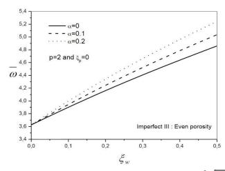
Fig. 19 Variation of the nondimensional fundamental frequency  $\overline{\omega} = \frac{\omega L^2}{h} \sqrt{\frac{\rho_m}{E_m}}$  of FG beam with Winkler parameter  $\xi_w$  and porosity coefficient  $\alpha$
