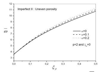
Fig. 22 Variation of the nondimensional fundamental frequency  $\overline{\omega} = \frac{\omega L^2}{h} \sqrt{\frac{\rho_m}{E_m}}$  of FG beam with shear foundation parameter  $\xi_p$  and porosity. coefficient  $\alpha$
