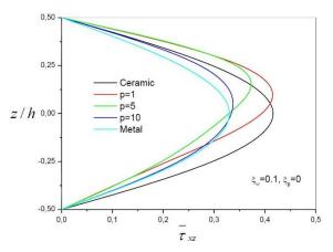
Fig. 12 Non-dimensional transverse shear stress through the thickness (L/h = 5, non-dimensional elastic foundation parameters are :  $\xi_w = 0.1$  and  $\xi_p = 0$ )
