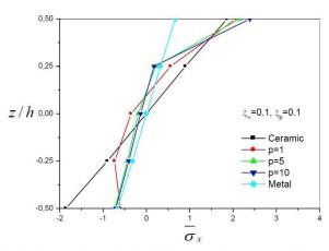
Fig. 10 Non-dimensional axial stress through the thickness (L/h = 5, non-dimensional elastic foundation parameters are :  $\xi_w = 0.1$  and  $\xi_p = 0.1$ )
