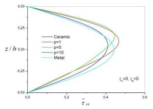
Fig. 11 Non-dimensional transverse shear stress through the thickness (L/h = 5, non-dimensional elastic foundation parameters are :  $\xi_w = 0$  and  $\xi_p = 0$ )
