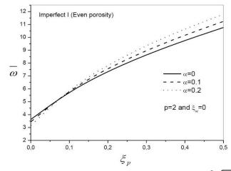
Fig. 21 Variation of the nondimensional fundamental frequency  $\overline{\omega} = \frac{\omega L^2}{h} \sqrt{\frac{\rho_m}{E_m}}$  of FG beam with shear foundation parameter  $\xi_p$  and porosity coefficient  $\alpha$
