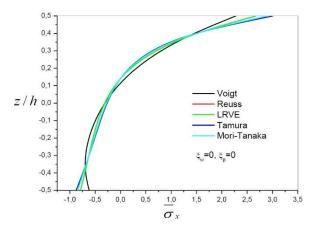
Fig. 14 Variation of the axial stress  $\overline{\sigma}_x$  through-the-thickness of a FG beam for different micromechanical models (L/h = 2, p = 1)
