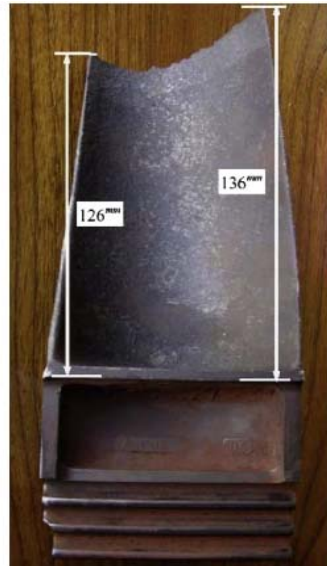
Fig. 5 the distances of the fracture surface from the platform blade edges (Poursaeidi et al. 2008)
