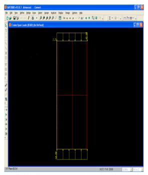
Fig. 2 Applied loadings on cement plastered typha strawbale wall
