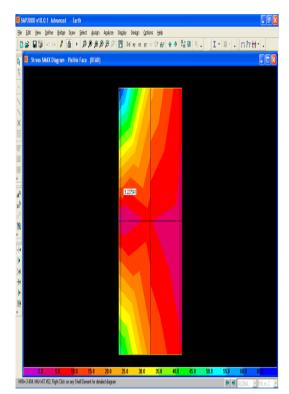
Fig. 8 Maximum stress diagram of earth plastered typha strawbale wall
