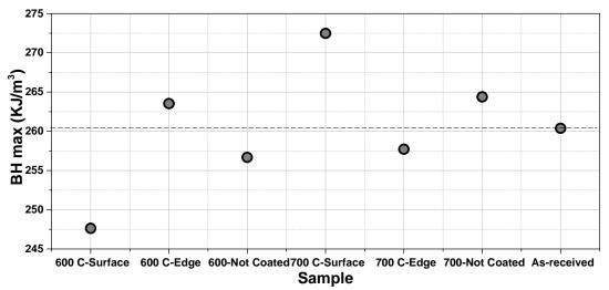
Fig. 3 Plot of energy product,  $BH_{max}$  vs. samples (after sputter deposition of Dy films onto both edges and whole surface of the magnet followed by post-annealing at 600 and 700 °C).
