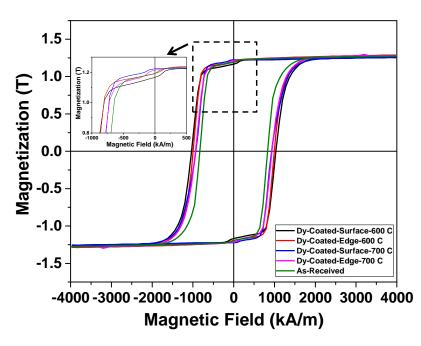
Fig. 2 Hysteresis loops after sputter deposition of Dy films onto both edges and whole surface of the magnet followed by post-annealing at 600 and 700  $^{\circ}$ C
