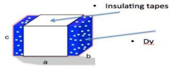
Fig. 1 Schematic of the N-38 Dy-free Neo magnet surfaces where Dy was sputter-coated onto the edges (other areas were masked).
