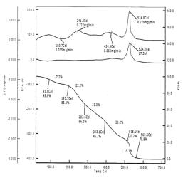
3(b) Thermogram Fig. of (gelatin-co-PVA)-g-poly (AAc) copolymer
