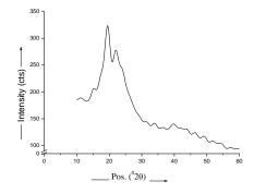
Fig.5(a) XRD pattern of the gelatin-co-PVA copolymer
