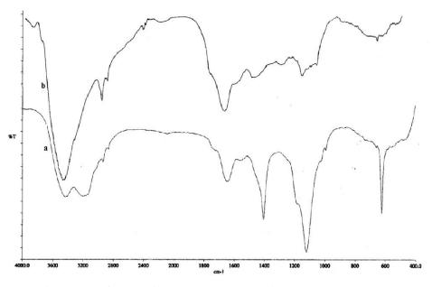
Fig. 2 FTIR of (a) gelatin-co-PVA and (b) (gelatin-co-PVA)-g-poly (AAc)
