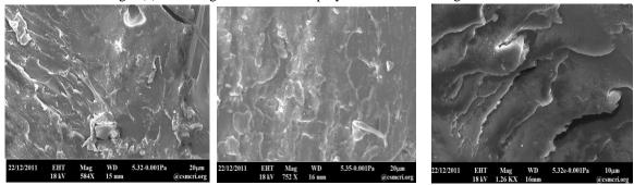
752 X 584 X 1.26 K X Fig.4 (b) SEM of (gelatin-co-PVA)-g-poly (AAc) copolymer at different magnifications
