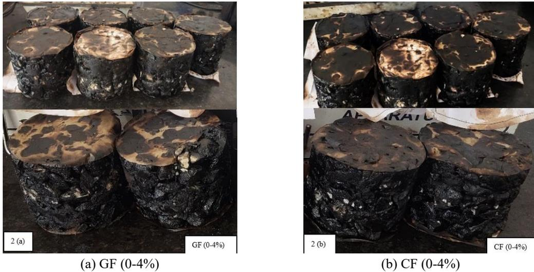
Fig. 2 Laboratory specimens using glass and carbon fiber with different percentages of fibers (0-4%)
