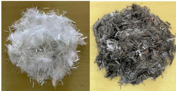
Fig. 1 Glass and carbon fiber used in this study
