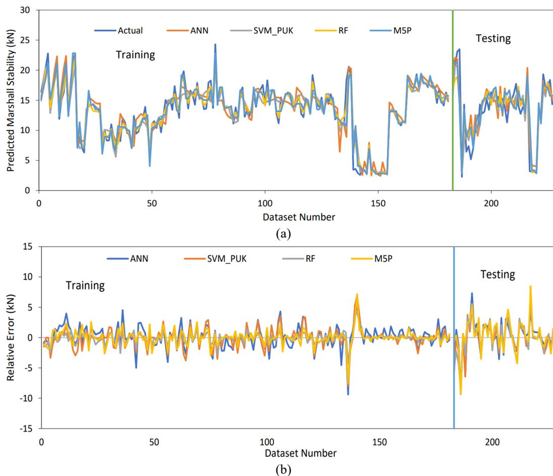
Fig. 14 Error graph between actual and predicted values using ANN, SVM\_PUK RF and M5P based models for training and testing stages
