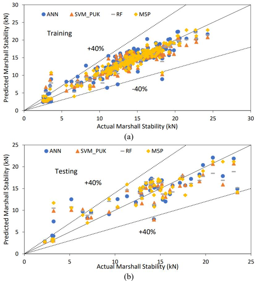
Fig. 12 Actual and predicted values using ANN, SVM\_PUK, RF and M5P Tree based models for training and testing stages
