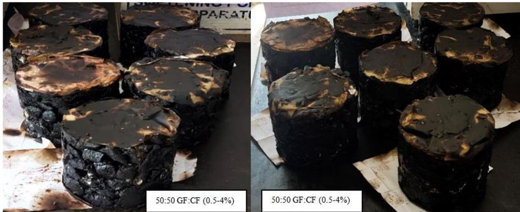
Fig. 3 Laboratory specimen in combination with glass and carbon fiber using different percentages of bitumen (0.5-4%)
