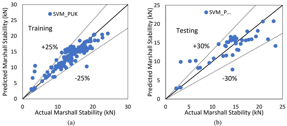
Fig. 9 Actual and predicted values using SVM\_PUK-based models for training and testing stages
