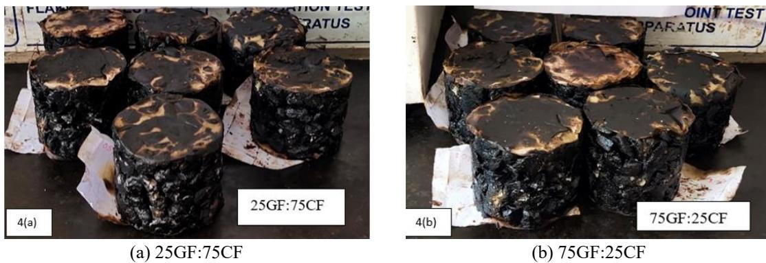
Fig. 4 Laboratory specimens (glass and carbon fiber) using bitumen (0.5-4%)
