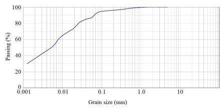
Fig. 2 The grain size analysis results for Tabriz landfill soil
