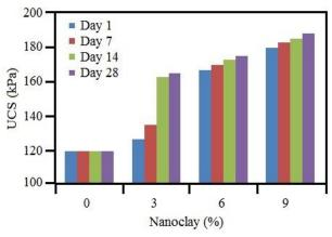
Fig. 5 The nanoclay content impact on UCS
