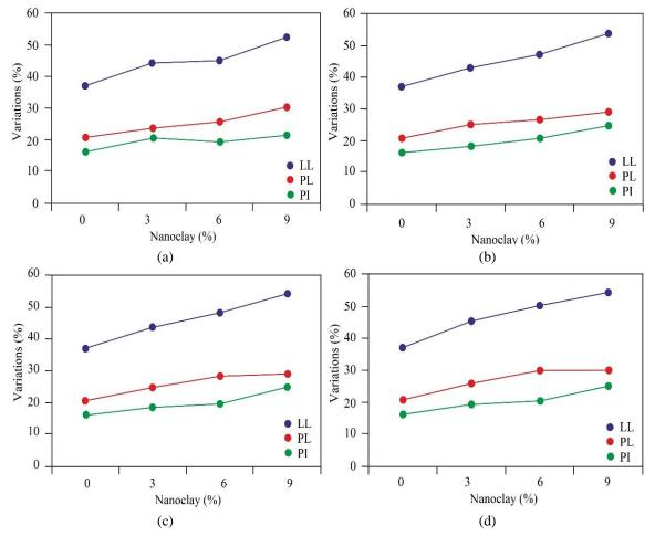
Fig. 3 Atterberg limits variation in soil based on nanoclay content (a) 1 day, (b) 7 day, (c) 14 day and (d) 28 day
