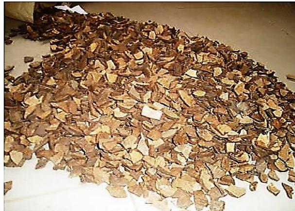
Fig. 2 Coconut shell as coarse aggregate (CSA) after crushing (Afolayan *et al.* 2017)
