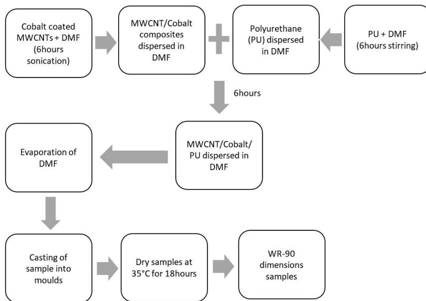
Fig. 3 Process of Composites: Cobalt coated MWCNTs/PU
