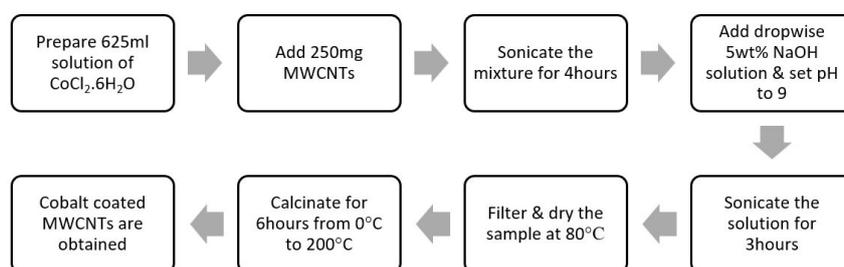
Fig. 2 Preparation of Cobalt coated MWCNTs
