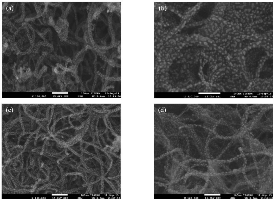
Fig. 4 FESEM of Cobalt coated MWCNTs with varying Cobalt composition (a) CMP 1; (b) CMP 2; (c) CMP 3; (d) CMP 4
