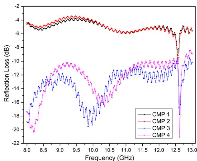
Fig. 6 Microwave absorption characteristics of the composites with varying compositions of Co/MWCNTs/PU
