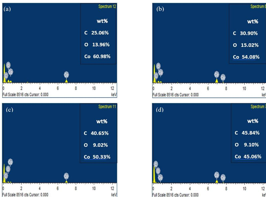
Fig. 5 EDX analysis of Cobalt coated MWCNTs with varying Cobalt composition (a) CMP 1; (b) CMP 2; (c) CMP 3; (d) CMP 4
