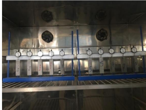
Fig. 4 Drying shrinkage specimens in a humidity chamber
