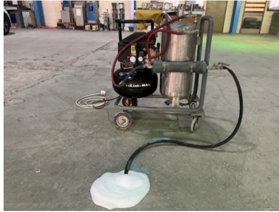
Fig. 1 Foam generator used in this study
