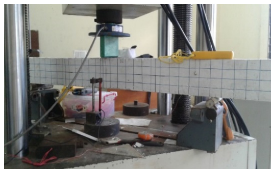
Fig. 6 Three-point bending test for RC beam
