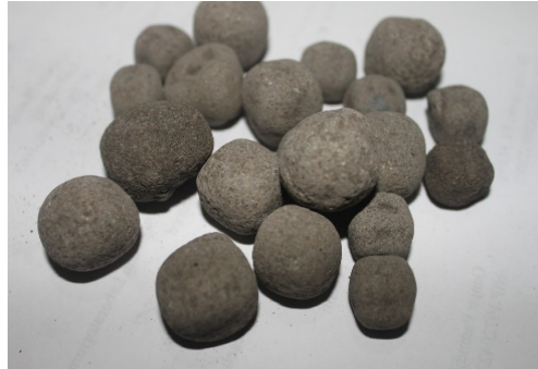
Fig. 3 Polypropylene waste coarse aggregate coated with sand
