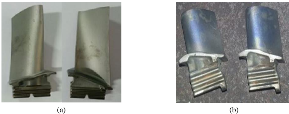
Fig. 2 Gas turbine blade (a) Before Heat treatment; (b) After Heat treatment
