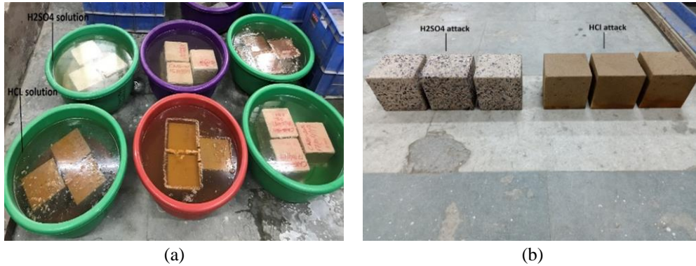
Fig. 6 Samples immersed in H 2 SO 4 and HCl solutions and its physical appearance after immersion
