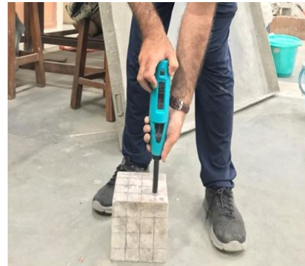
(b) Rebound hammer reading
