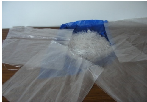
Fig. 1 Woven bags and recycled polypropylene fiber (RPF) used
