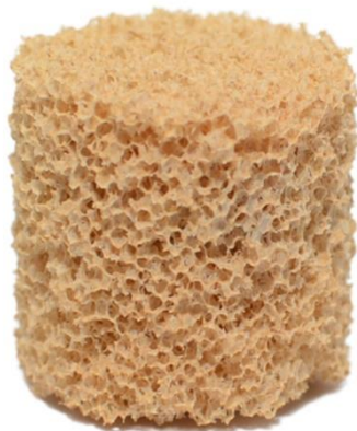
Fig. 1 A porous composite support catalyst made from clay and fly ash
