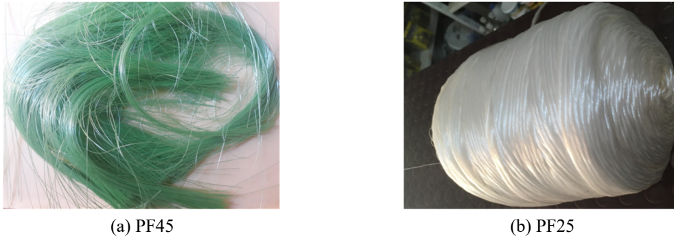
Fig. 1 Natural look of the used polypropylene fibers
