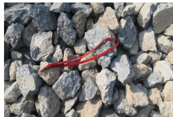
Fig. 2 Hammer crushed boulders
