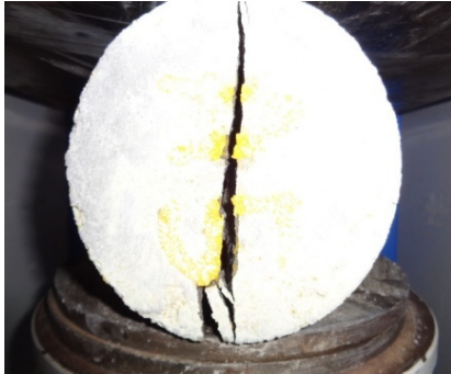
Fig. 5 Split tensile strength test set up
