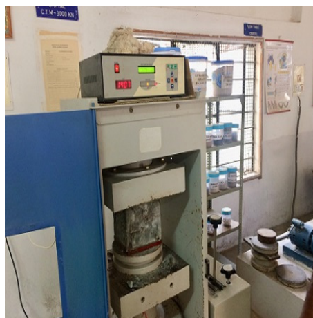
Fig. 4 Cube compressive strength test set up
