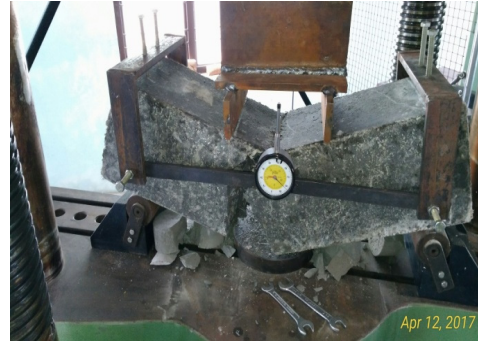
Fig. 6 Flexural strength test set up
