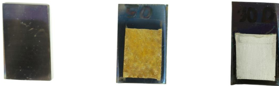
(a) As-received specimen (b) AC-anodized specimen (c) DC-anodized specimen
