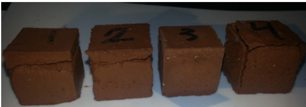
Fig. 3 Visual observation of CW activated by different NaOH & Na 2 SiO 3 content after 24h of water curing
