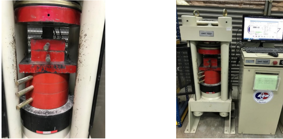
Fig. 8 Compressive strength test instrument (compression machine with 3000 kN capacity)
