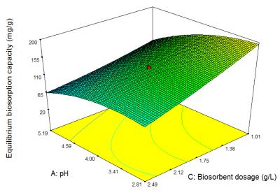
Fig. 2 Response surface plot indicating the effect of pH and biosorbent dosage on the metal uptake (q)
