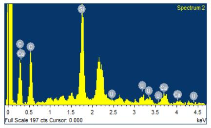
Fig. 9 EDX analysis of uranium bounded to the S. boveanum surface
