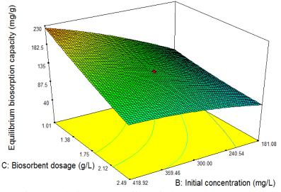
Fig. 3 Response surface plot indicating the effect of biosorbent dosage and initial uranium ion concentration on the metal uptake (q)
