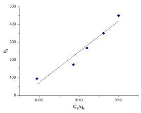
Fig. 4 Langmuir isotherm of uranium biosorption by S. boveanum
