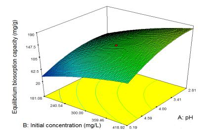
Fig. 1 Response surface plot indicating the effect of pH and initial uranium ion concentration on the metal uptake (q)
