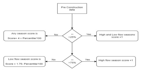
Fig. 2 Working flow chart of high and low flow seasons (\*\*The percentile values are fixed based on the Post construction period data)
