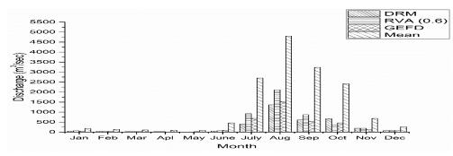
Fig. 5 Comparison of MAF with three different Hydrological methods for Srisailam
