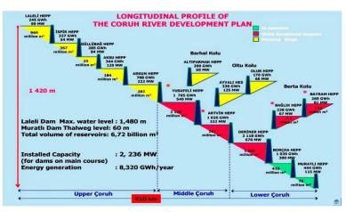
Fig. 1 Longitudinal profile of the Coruh River development plan
