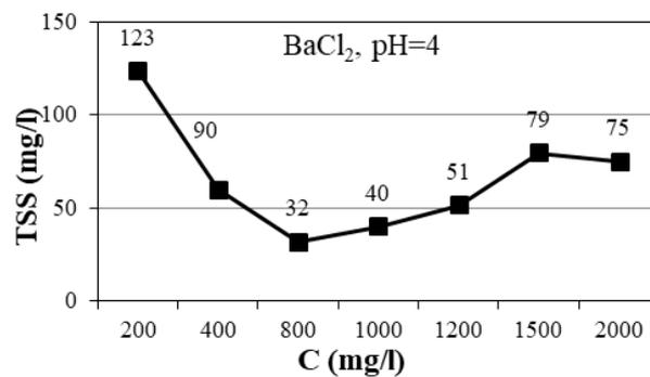
Fig. 11 The effect of changing BaCl<sub>2</sub> concentration on the TSS removal at pH=4
