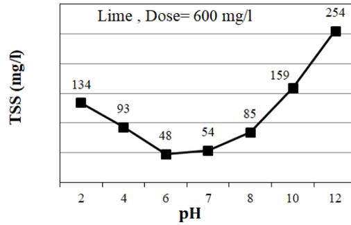
Fig. 3 The effect of changing pH on removal of TSS using 600 mg/l lime
