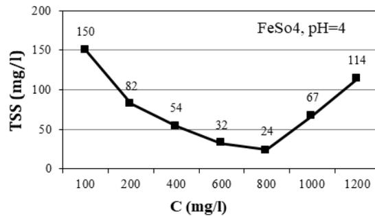
Fig. 9 The effect of changing FeSO<sub>4</sub> concentration on the TSS removal at pH=4
