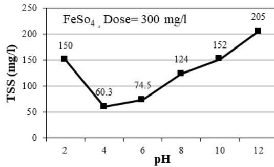
Fig. 8 The effect of changing pH on TSS removal using 300 mg/l FeSO<sub>4</sub>
