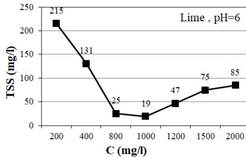
Fig. 4 The effects of changing lime concentration on TSS removal at pH=6 at TSS removal
