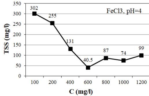
Fig. 7 The effects of changing FeCl<sub>3</sub> concentration on TSS removal at pH=4
