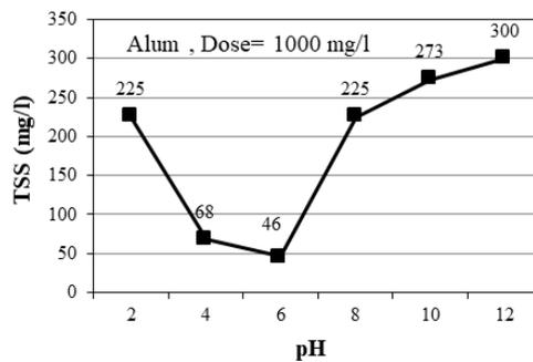
Fig. 1 The effect of changing pH on TSS removal using 1000 mg/l Alum
