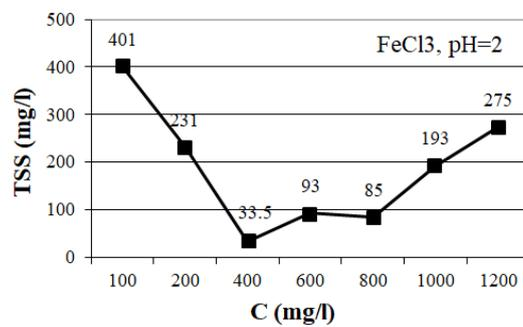
Fig. 6 The effects of changing FeCl<sub>3</sub> concentration on TSS removal at pH=2
