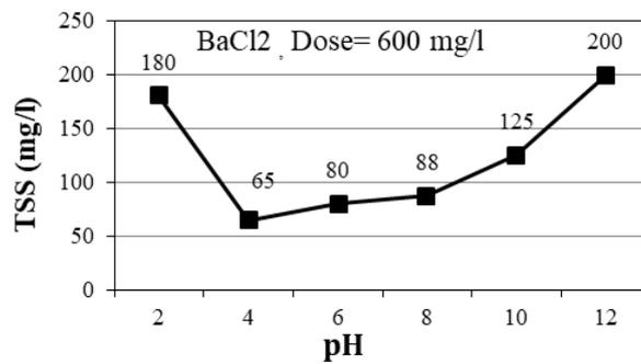
Fig. 10 The effect of changing pH 4 on TSS removal using 600 mg/l BaCl<sub>2</sub>
