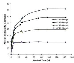
Fig. 2 Effect of initial AY36 concentration on adsorption capacity of RTAC (V=100 ml,  $C_o=20-80$  mg/l, Adsorbent dose=0.1 g, pH=6.5±0.5, Temperature=29±1°C)
