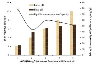
Fig. 3 Effect of pH on adsorption capacity of RTAC (V=100 ml,  $C_o$ =80 mg/l, Adsorbent Dose=0.1 g, pH (2-10), Temperature=29±1°C)
