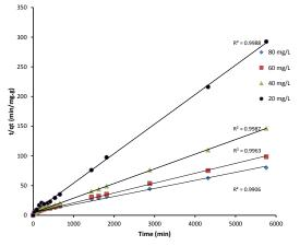
Fig. 7 Pseudo-second-order kinetics for adsorption of AY36 on TAC at 29±1°C
