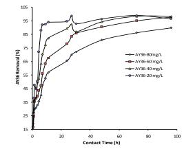
Fig. 1 Initial AY36 concentration and removal by RTAC (V=100 ml,  $C_o=20-80$  mg/l, Adsorbent Dose=0.1 g, pH=6.5±0.5, Temperature=29±1°C)
