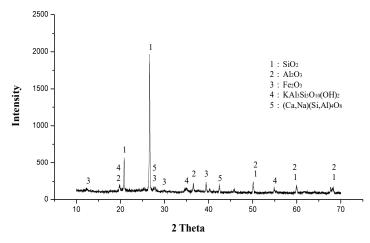
Fig. 2 Crystal structure analysis of the sludge by X-ray diffraction (XRD)
