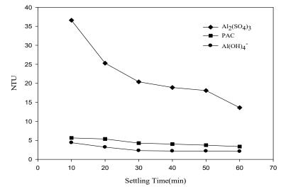
Fig. 8 Supernatant turbidity of synthesized solutions treated by Al<sub>2</sub>(SO<sub>4</sub>)<sub>3</sub>, PACl, and Al(OH)<sub>4</sub><sup>-</sup>
