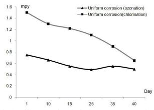
Fig. 3 Uniform corrosion plot in the two treatment methods
