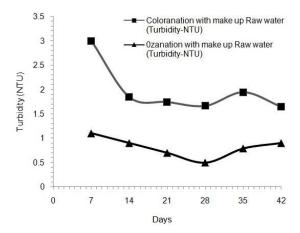
Fig. 6 Turbidity plot in the two treatment methods
