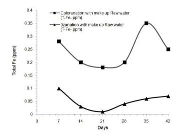
Fig. 7 Soluble Fe plot in the two treatment methods
