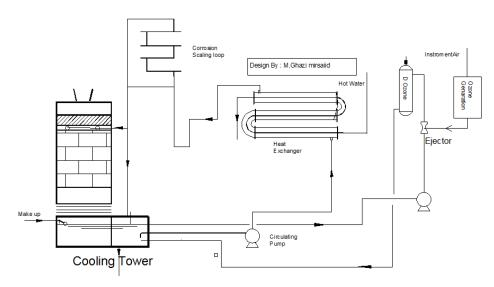
Fig. 1 Block diagram for the ozone treatment pilot plant
