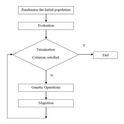
Fig. 4 Typical GP flowchart
