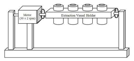
Fig. 2 Rotary extraction apparatus for the leachability experiments
