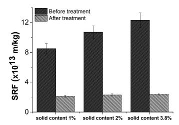
Fig. 3 Effect of different sludge solids content on the SRF of the sludge after treatment with *A*. *ferrooxidans* and *A. thiooxidans* (AF+AT)
