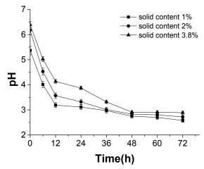
Fig. 1 Effect of different sludge solids content on the bioacidification during treatment with *A*. *ferrooxidans* and *A. thiooxidans* (AF+AT)
