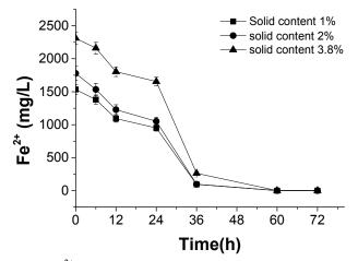
Fig. 2 Bio-oxidation of  $Fe^{2+}$  in sludge with different solids content with time during the treatment with *A. ferrooxidans* and *A. thiooxidans* (AF+AT)
