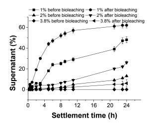
Fig. 4 Effect of different sludge solids content on supernatant removal after treatment with *A*. *ferrooxidans* and *A. thiooxidans* (AF+AT)
