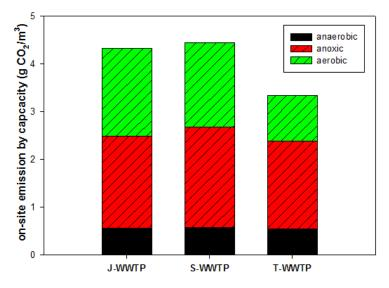
Fig. 3 The total on-site GHG emissions from anaerobic, anoxic, and aerobic process at three different WWTPs
