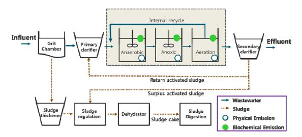
Fig. 1 Flow diagram of hybrid WWTP and system boundary for the estimation of GHG emissions
