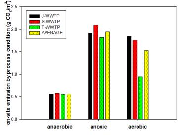
Fig. 4 On-site GHG emissions at different process conditions
